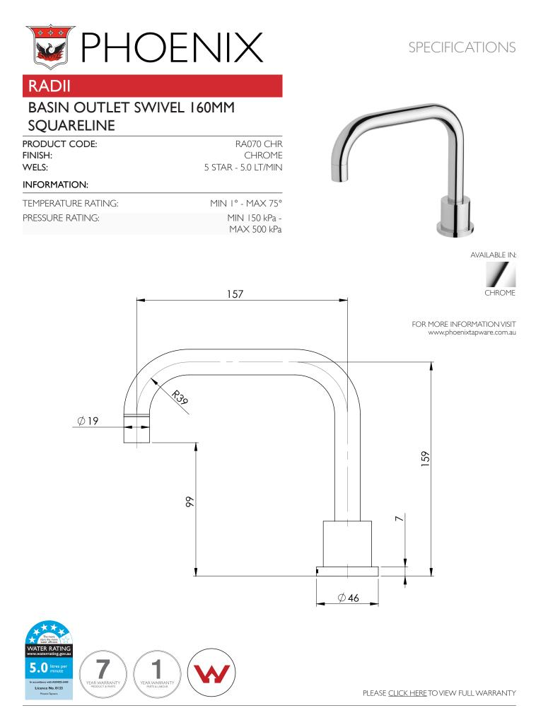
While we aim to ensure the specifications shown are correct at time of printing. Phoenix Tapware reserves the right to make modifications without prior notice. Always use the physical product measurements for mark-ups and roughing-in as the line drawing shown may differ from the actual product over time. All measurements are shown in millimetres.
